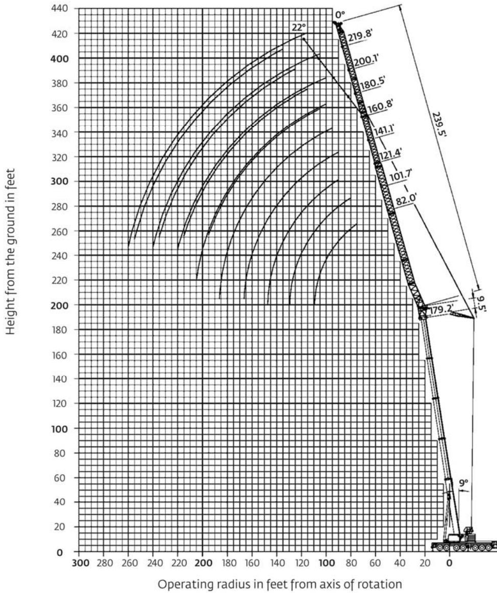
*Hook heights shown in the working diagram do not consider loaded boom deflection.*
