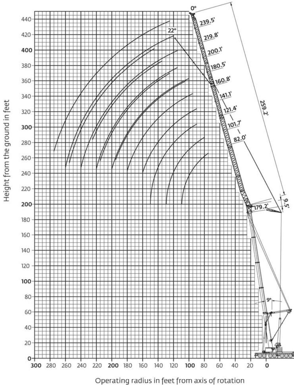
*Hook heights shown in the working diagram do not consider loaded boom deflection.*
