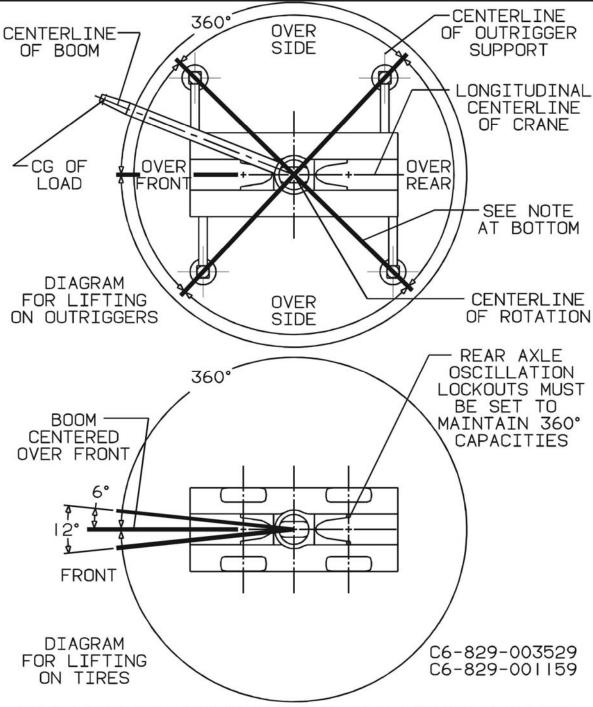
BOLD LINES DETERMINE THE LIMITING POSITION OF ANY LOAD FOR OPERATION WITHIN WORKING AREAS INDICATED WORKING AREA DIAGRAM
