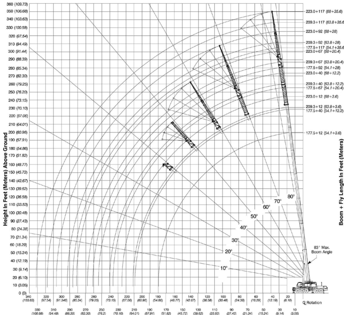
Operating Radius From Centerline of Rotation In Feet (Meters)
