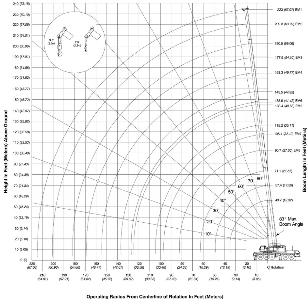
Operating Radius From Centerline of Rotation In Feet (Meters)
